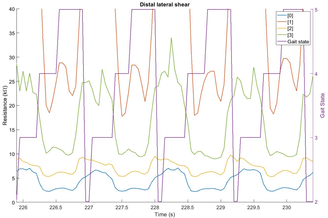
Figure 3: Four directions (0-3) of distal lateral shear stress during level ground walking at self-selected walking speed. Gait states: 2 = toe-off; 3 = swing phase; 4 = heel strike; 5 = stance phase.
