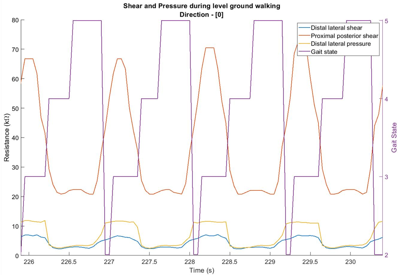
Figure 2: Shear and pressure measurements during level ground walking at self-selected walking speed. Gait states: 2 = toe-off; 3 = swing phase; 4 = heel strike; 5 = stance phase.
