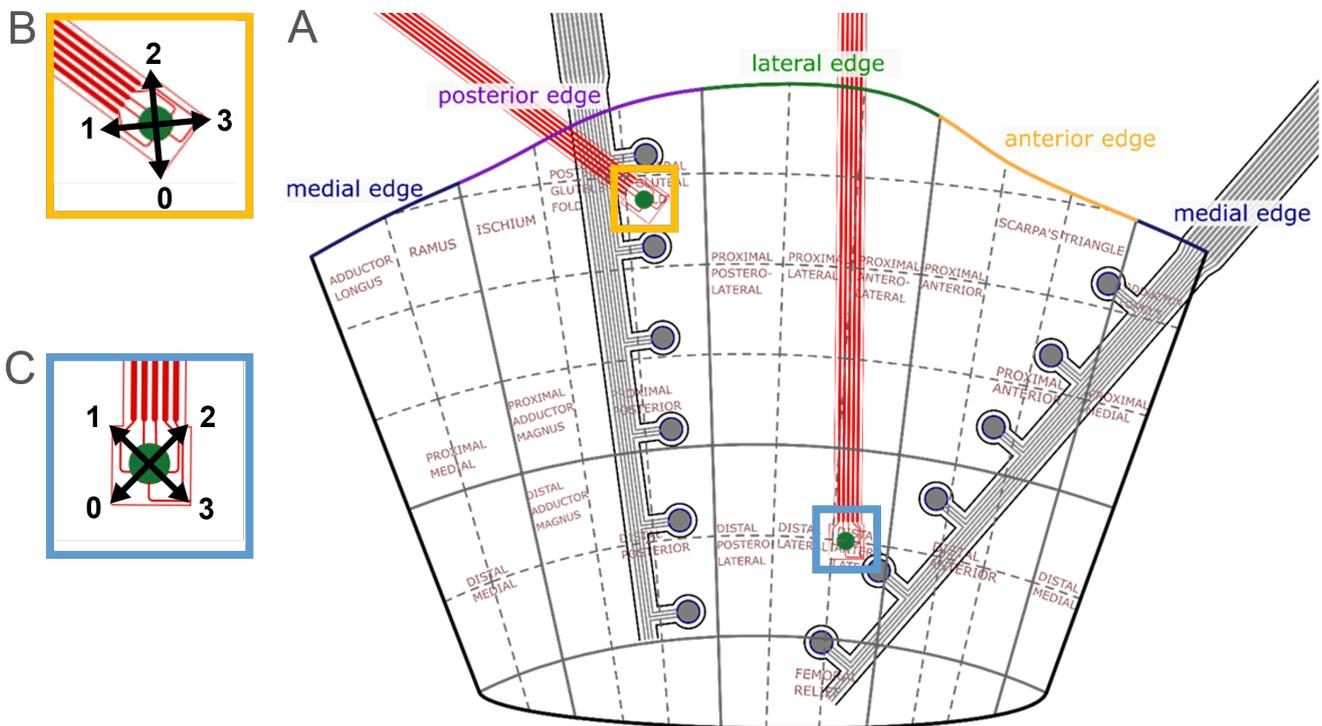
Figure 1 (A): Shear and pressure sensor positions on a 2D representation of the test subject's residual limb. Shear sensor measurement directions at proximal posterior (B), and distal lateral (C).
