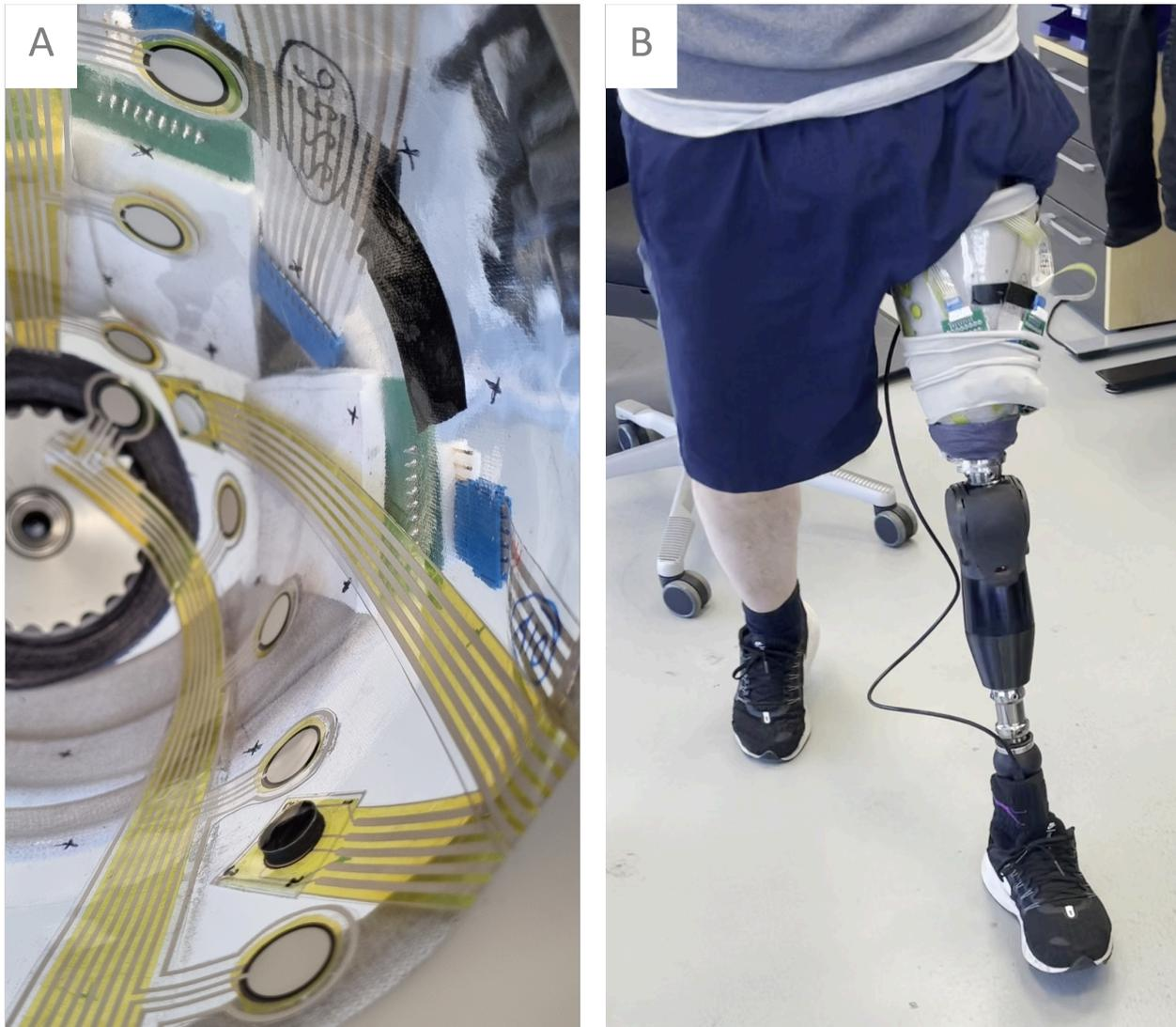
*Figure 4 (A): Printed shear and pressure sensors integrated inside socket. (B): Test subject wearing prosthesis with sensors integrated in a transparent replica socket.*
