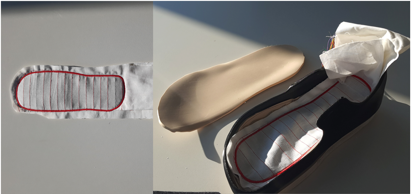
Image: Image 3 Prototype consisting of embroidered pressure sensors and commercial temperature sensors_182.png
